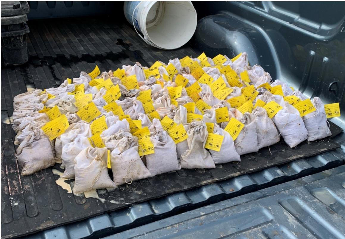
Figure 6-3. Bagged drill cuttings (source: DBS&A).
