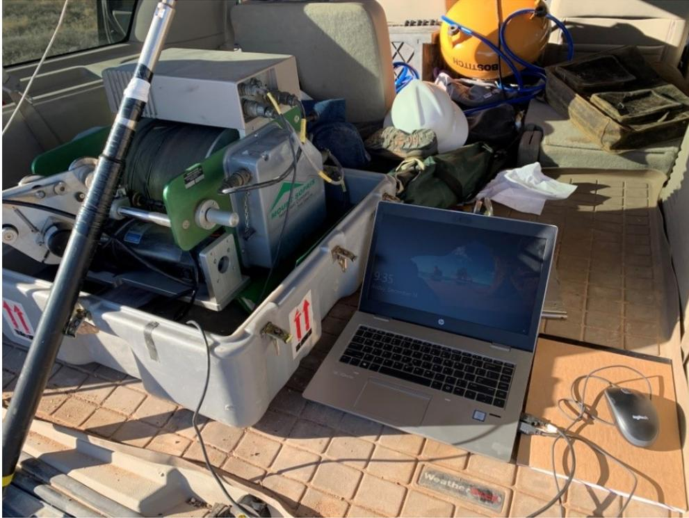
Figure 7-3. Geophysical logging data acquisition system.
