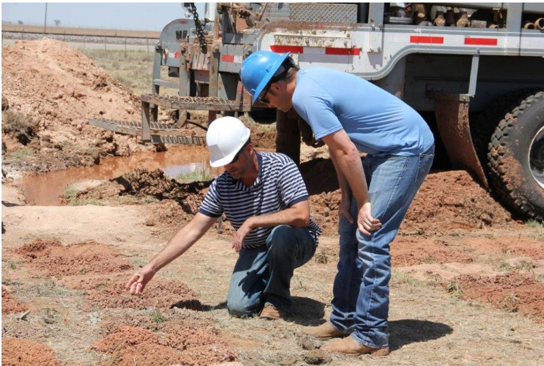
**Figure A-3. Examining exploratory test boring drill cuttings.**
