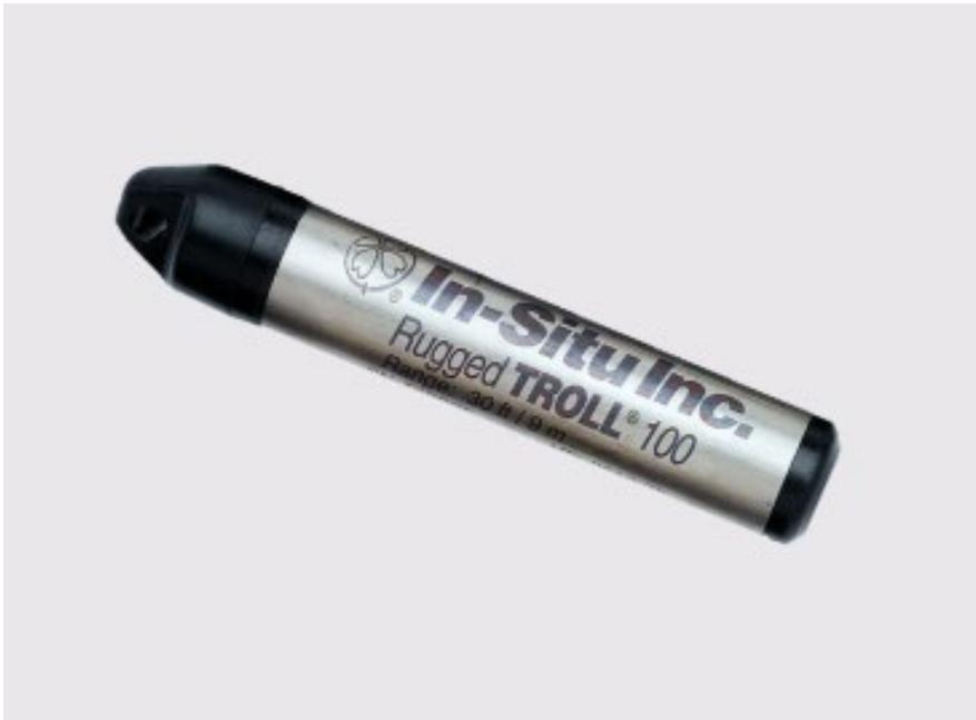
Figure 8-4. Self-contained pressure transducer with built-in data logger. Suspension cable not shown. This type of transducer must be removed from the well in order to retrieve the recorded data (source: In-Situ, 2021).
