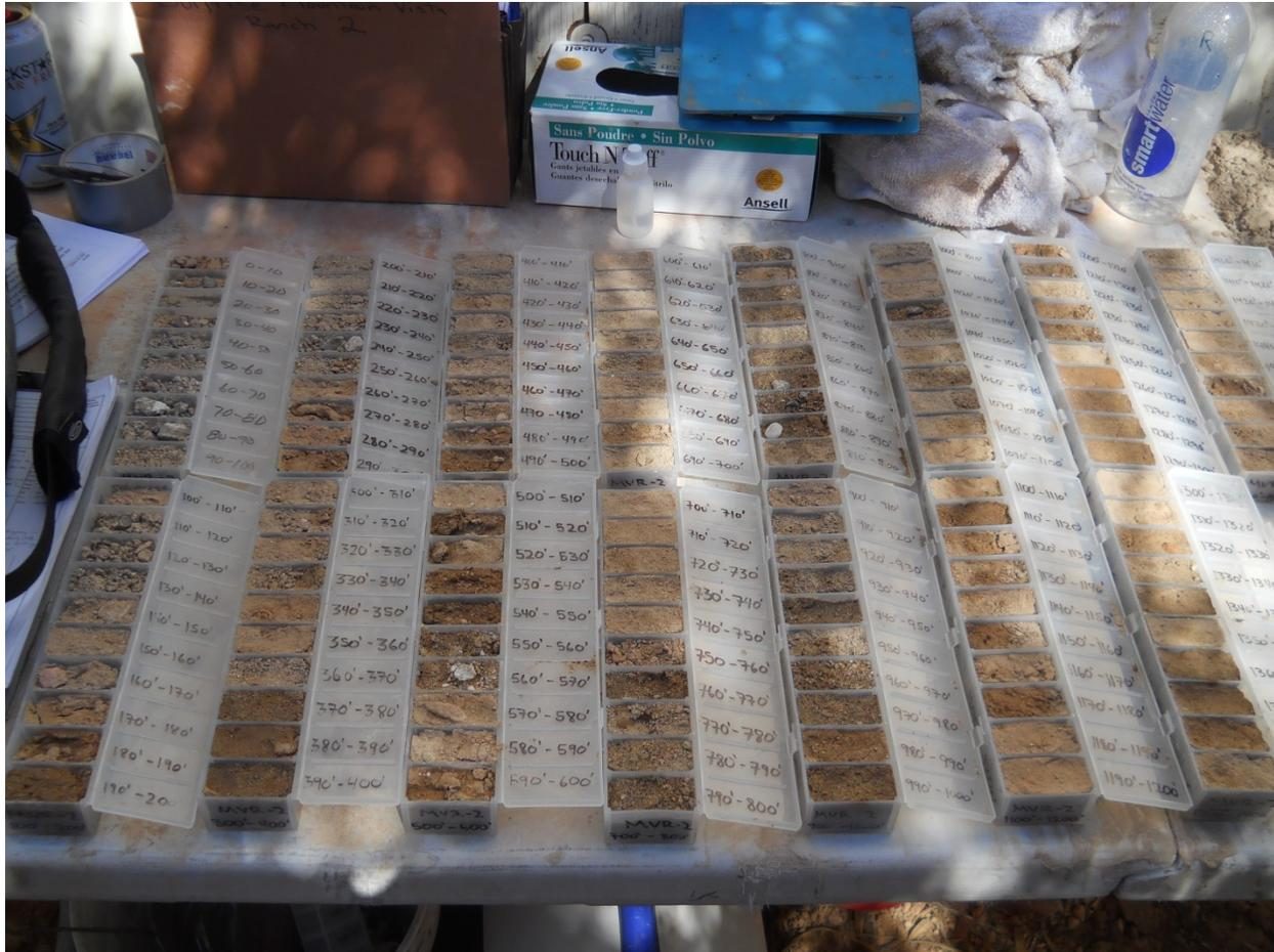
Figure 6-4. Drill cutting trays laid out for examination by the on-site geologist (source: DBS&A).
