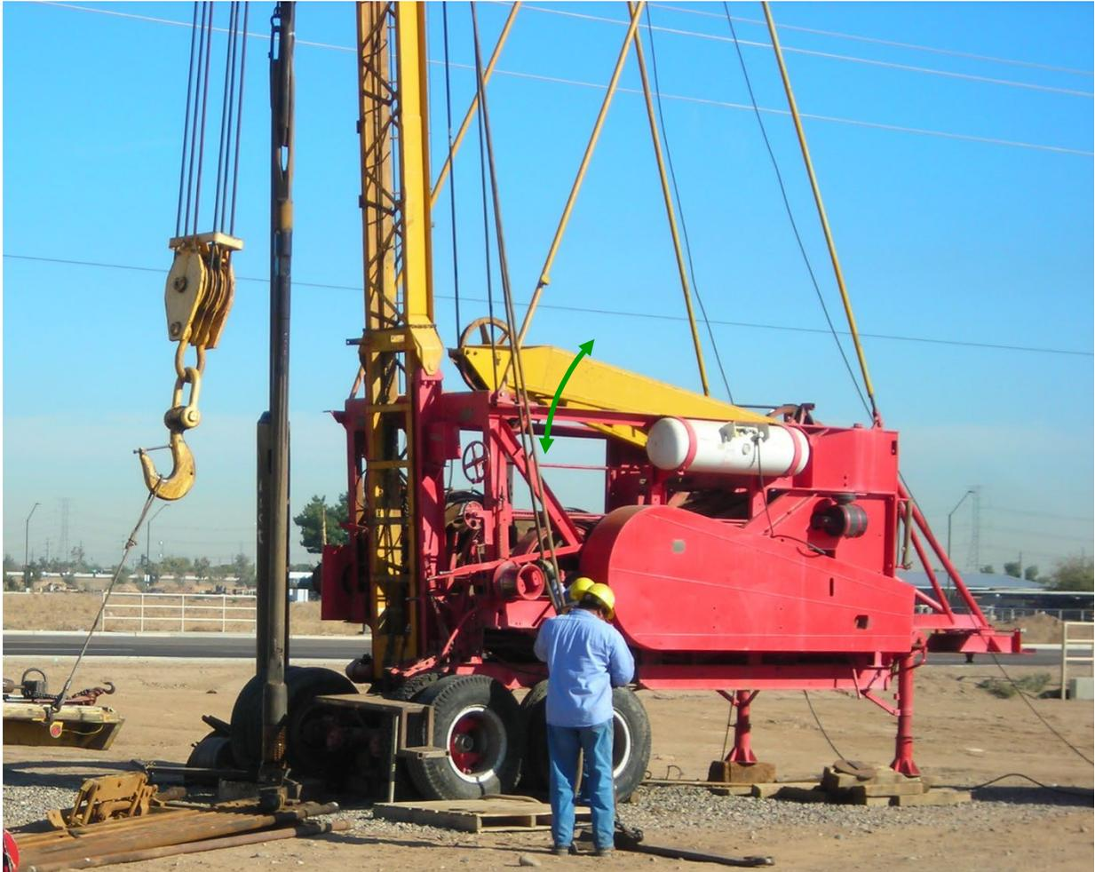
**Figure 3-10. Cable tool drilling rig (source: Clear Creek Associates). The walking beam (yellow) moves up and down (green arrow), which provides the motion of the drill cable. The drill string standing to the left of the rig includes the drill bit (at the base), drill string, and drilling jars (at the top of the photograph).**
