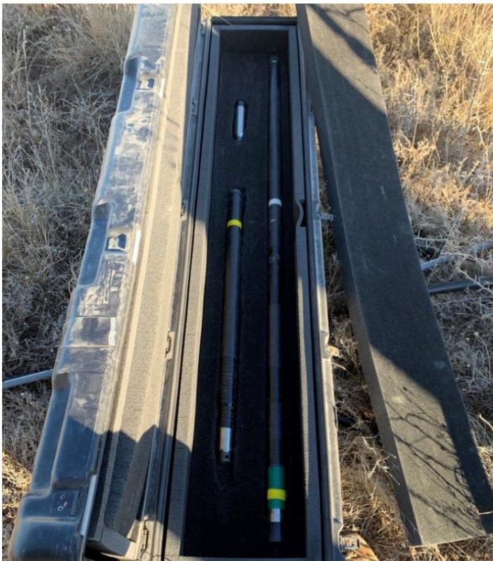
Figure 7-4. Geophysical logging tools.
