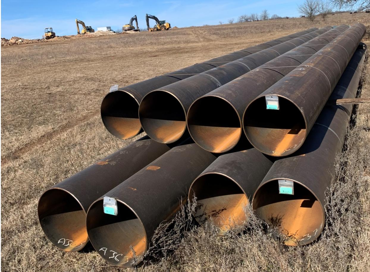
**Figure 3-14. 20-inch surface casing.**
