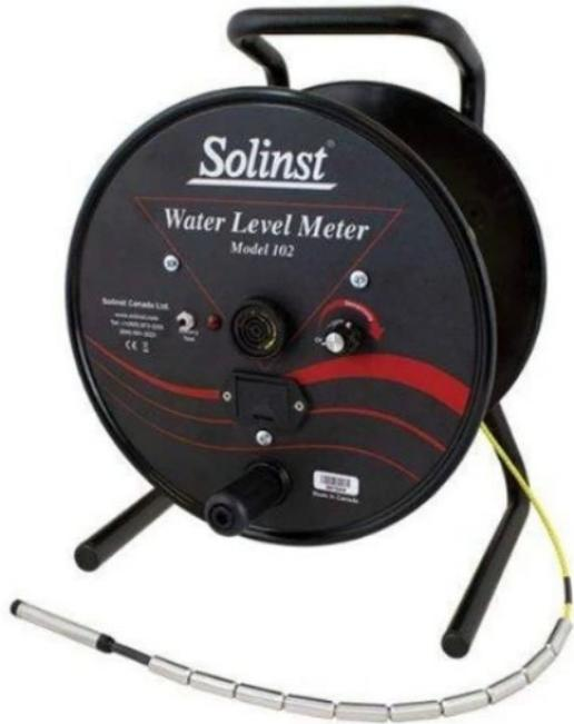
**Figure 8-2. Electronic water meter. The probe is lowered down the well until the water level is reached, at which point the alarm (beeping noise) will be triggered (source: Solinst, 2021).**
