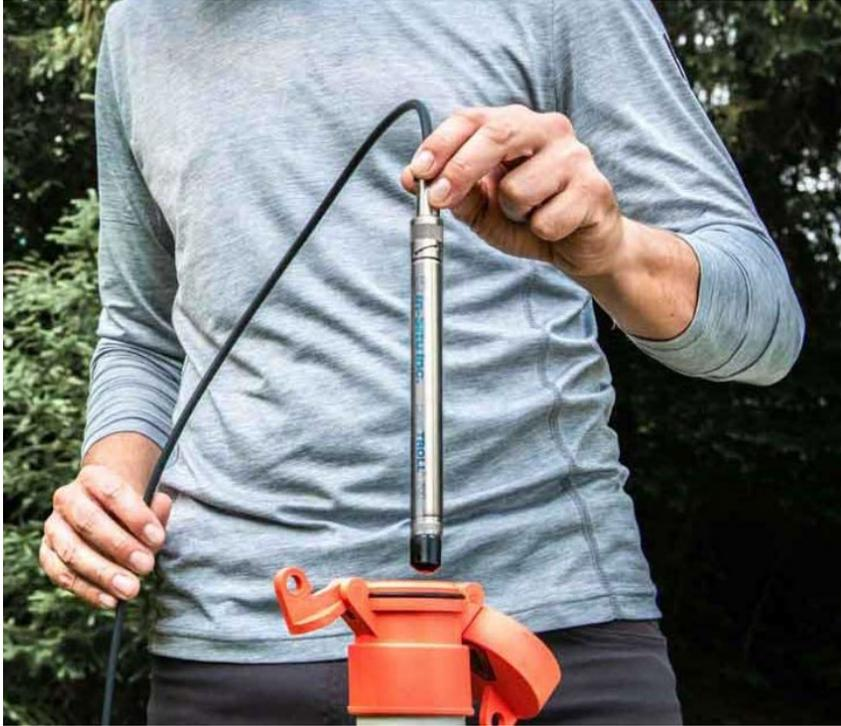
Figure 8-3. Pressure transducer with data cable being installed in a shallow monitor well (source: In-Situ, 2021).
