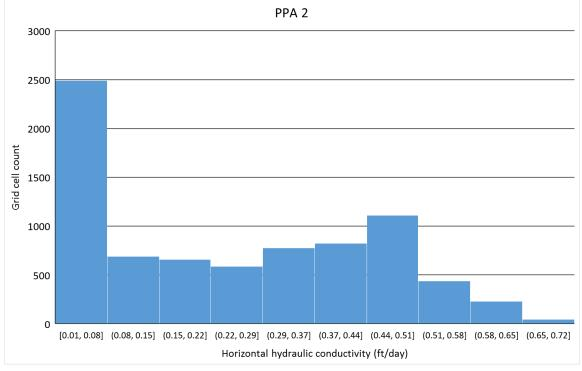
Figure 9-2.Rustler GAM calibrated horizontal hydraulic conductivity (feet per day) for PPA-2.Note: PPA=potential production area; ft/day=feet per day.
