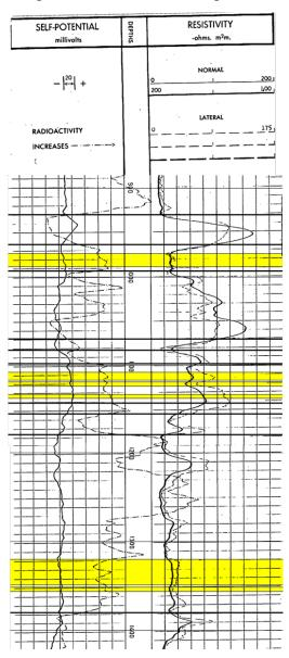
Figure 13-12. Example geophysical log used in additional calculations of total dissolved solids. Yellow highlights indicate areas where water quality was calculated.
