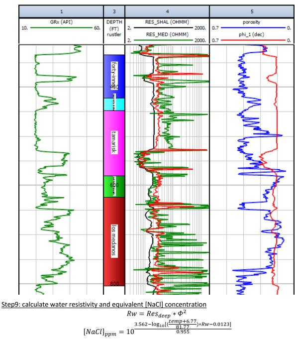
Since the equation above is derived from Archie's equation, it is only valid in clean intervals (shale free  $\Leftrightarrow$  local minimum of Gamma Ray signal). This means that we should do some truncations when calculating mean porosity and mean [NaCI] values.
