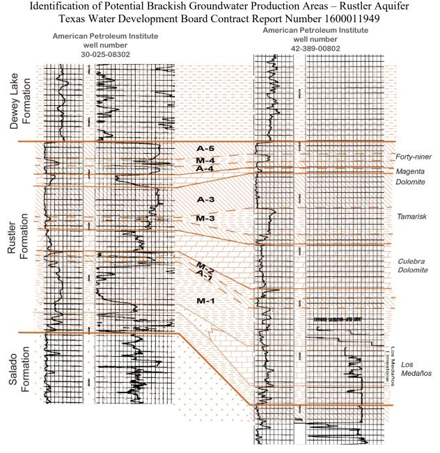
Figure 5-1. Two type logs form the northern and central portion of the Rustler Aquifer extent used to show how the specific geophysical log signatures relate to the Member and informal submember units of the Rustler Formation.
