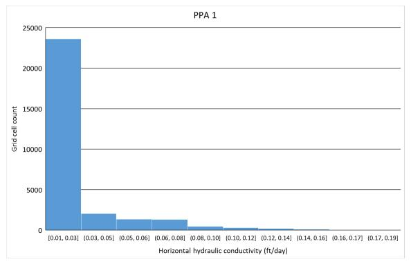
Figure 9-1. Rustler GAM calibrated horizontal hydraulic conductivity (feet per day) for PPA-1.
