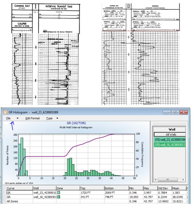
Figure 13-4. Example logs (423890108000 and 423893012000) for the gamma ray normalization process.
