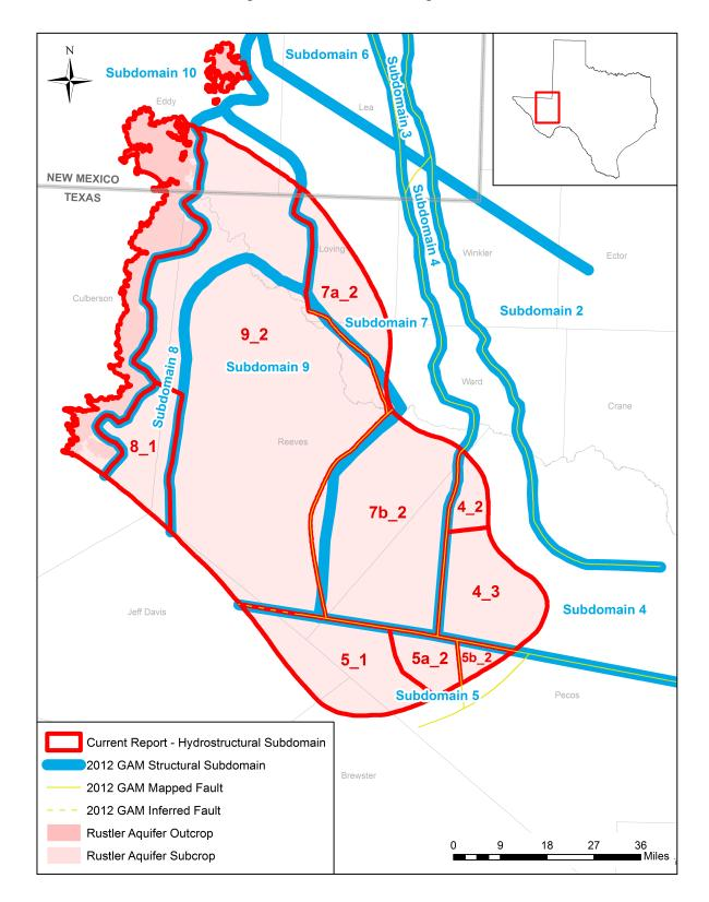
Figure 19-2. Hydrostructural subdomains used in the current report compared to the structural subdomains mapped in the original Rustler Groundwater Availability Model (GAM) (Ewing and others, 2012).
