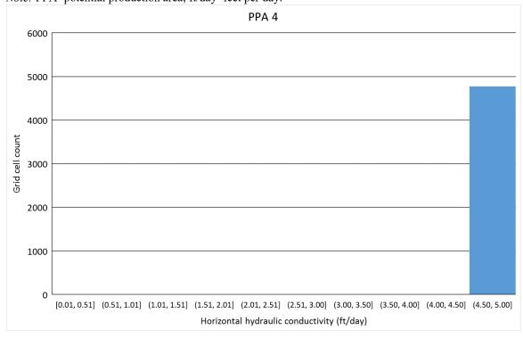
Figure 9-4.Rustler GAM calibrated horizontal hydraulic conductivity (feet per day) for PPA-4.Note: PPA=potential production area; ft/day=feet per day.
