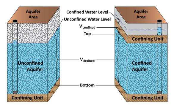
Figure 12-1. Schematic graph showing the difference between unconfined and confined aquifers (from Boghici and others, 2014).
