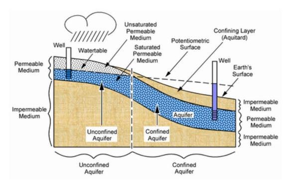
Figure 12-2. Schematic of aquifer transitioning from an unconfined outcrop region, where recharge from precipitation occurs, to confined conditions in the down dip regions of the aquifer (from Hermance, 2016).
