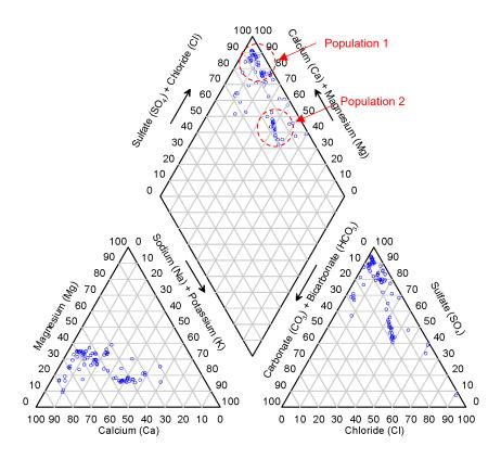
Figure 10-4. Piper plot of water chemistry analyses from wells producing from the Rustler Aquifer.
