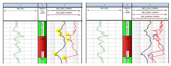
Figure 13-3. Example of depth shifting logs to better match between the resistivity signatures.
