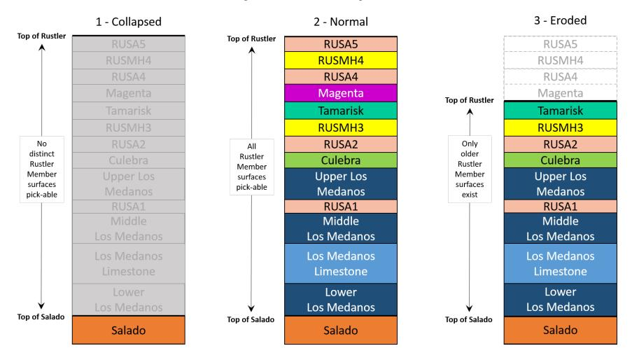
Figure 19-1. INTERA classification of stratigraphic columns from interpreted well logs for the creation of stratigraphy zones and volumetric regions.
