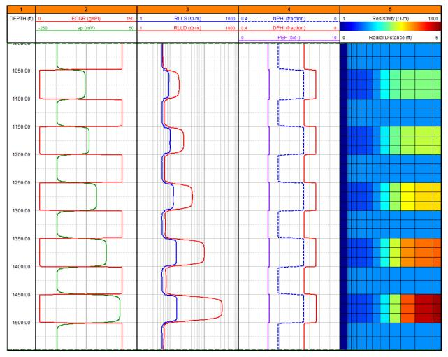
Figure 13-2. Example sensitivity analysis simulation showing a dolomitic unit straddled above and below by low resistivity shales.
