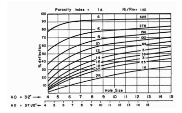
Figure 13-8. Graph used to calculate porosity from percent deflection and borehole diameter (Hilchie, 1984).
