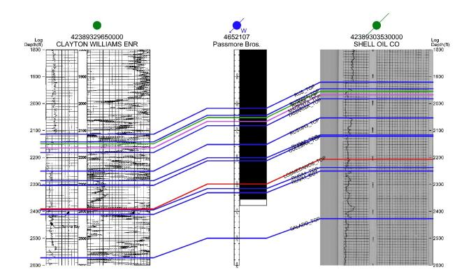
Figure 10-2. Example of how wells were evaluated to determine if completion was in the Rustler Aquifer.
