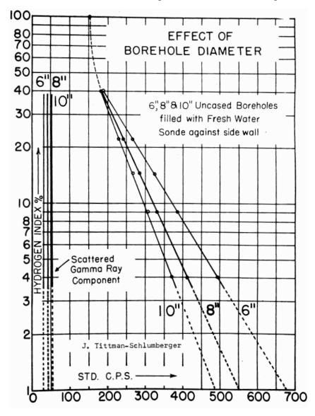
Figure 13-6 Calibration curve for a conventional neutron log to convert from Standard Counts Per Second (STD CPS) to Neutron Porosity Units (Hilchie, 1984)
