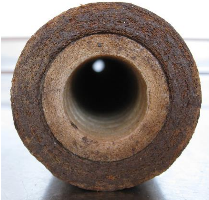
Figure 2. End of cartridge filter, note the light brown discoloration of the interior.
