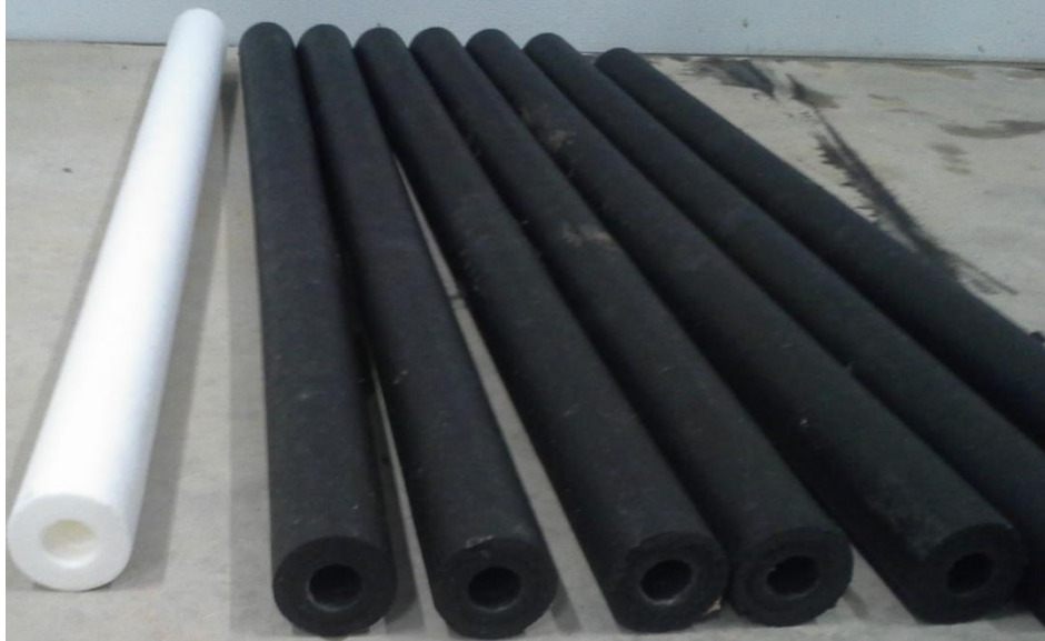
Figure 29. Prefilters removed on January 13, 2014 (new cartridge on left for comparison)
