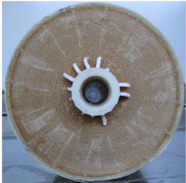
Figure 5. Concentrate-end of element F5375550.
