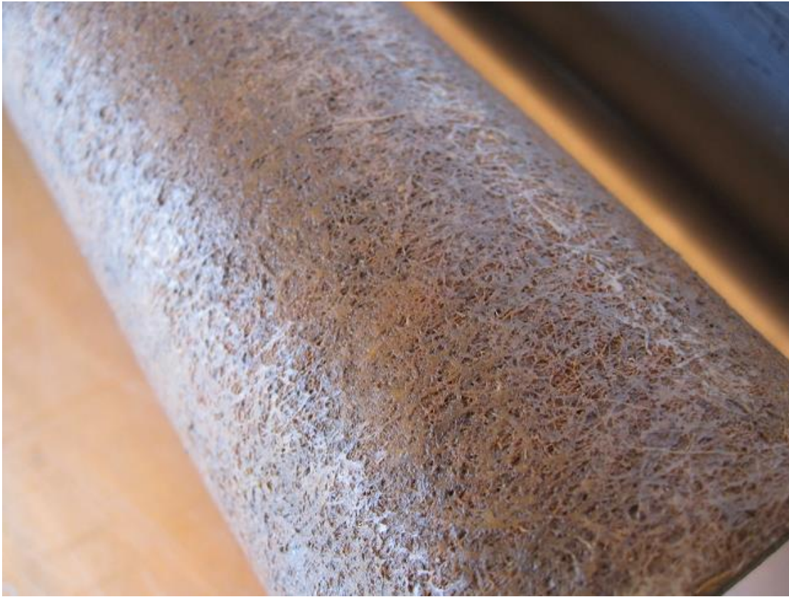
Figure 3. Close-up of cartridge filter surface, note the heavy coating of brown foulant.
