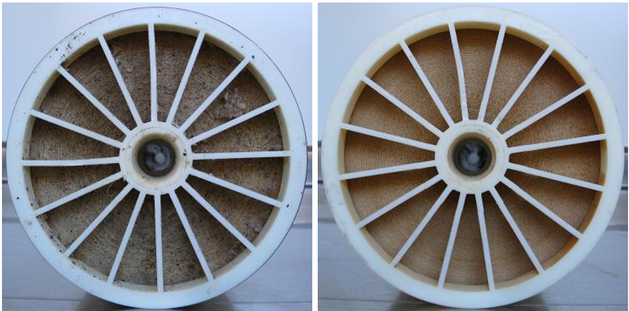
Figure 2. Feed-end of element F5375550, note the foulant build-up.
