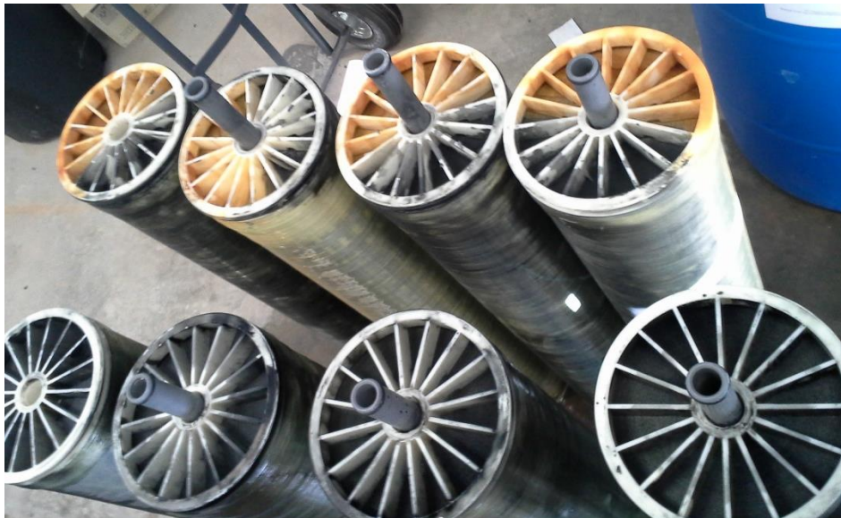
Figure 30. Membrane elements removed on January 13, 2014 (upper row Array 2, lower row Array 1)
