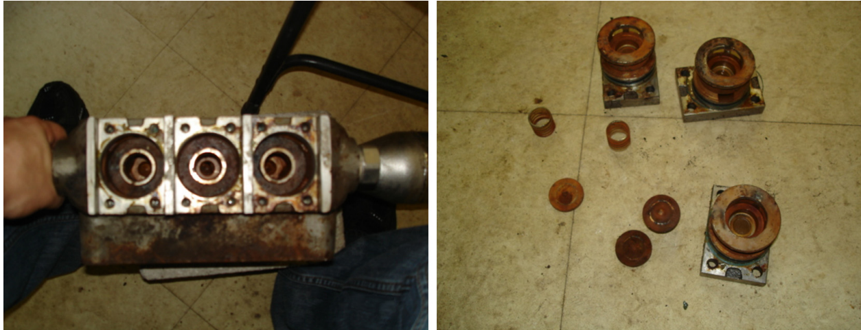
Figure II-31: Disassembled HPP showing check valves (left), disassembled HPP check valve (right).
