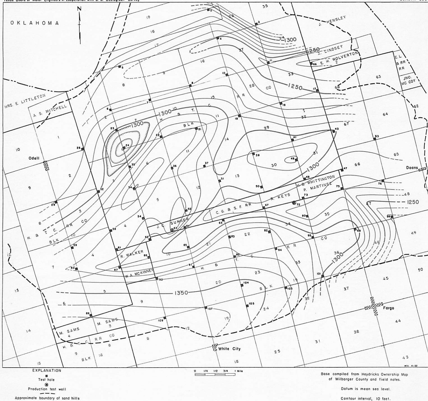
FIGURE 4.-Map showing contours on the Permian rocks beneath the Odell sand hills.
