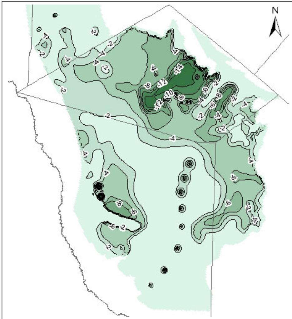
Figure 13. Difference in drawdowns in the Igneous aquifer after 50 years of pumping when using average compared to drought-of-record recharge. Water levels are lower, and therefore drawdowns are greater, throughout most of the aquifer area. However, except in the mountainous portions of the Davis Mountains, where no pumpage is located, the difference between average and drought-of-record recharge is less than 10 feet. Contour interval is 2 feet.
