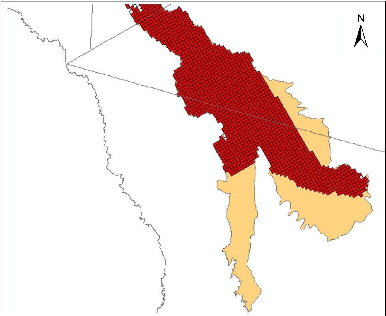
Figure 3. Extent of the Salt Basin aquifer in the GAM. Model cells in red are active cells that contain pumpage in 2000. Model cells in white are active cells without pumpage. The actual extent of the Salt Basin aquifer is shown in tan.
