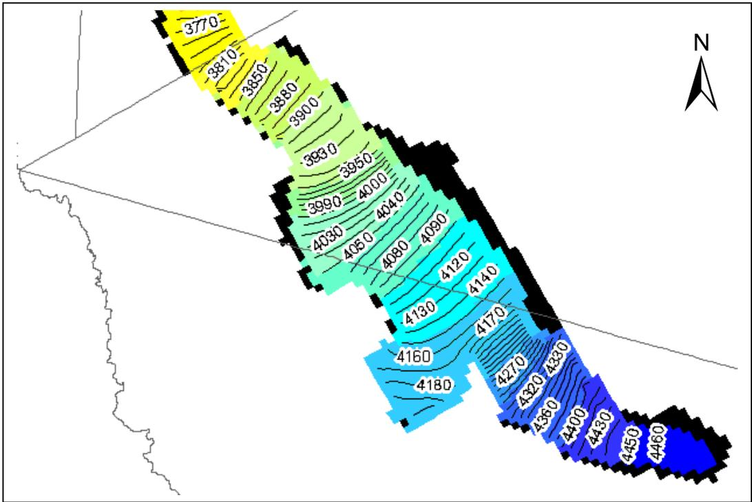
Figure 5. Water levels in the Salt Basin aquifer after 50 years of pumping using the 2000 estimated pumpage with average recharge. Contour interval is 10 feet. Dry model cells in the model run are shown in black.
