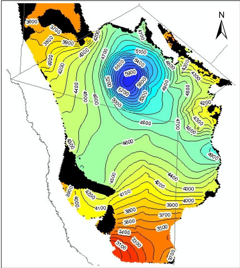
Figure 9. Initial water levels in the Igneous aquifer in the year 2000. Contour interval is 100 feet. Black areas are where the GAM showed the aquifer is dry.
