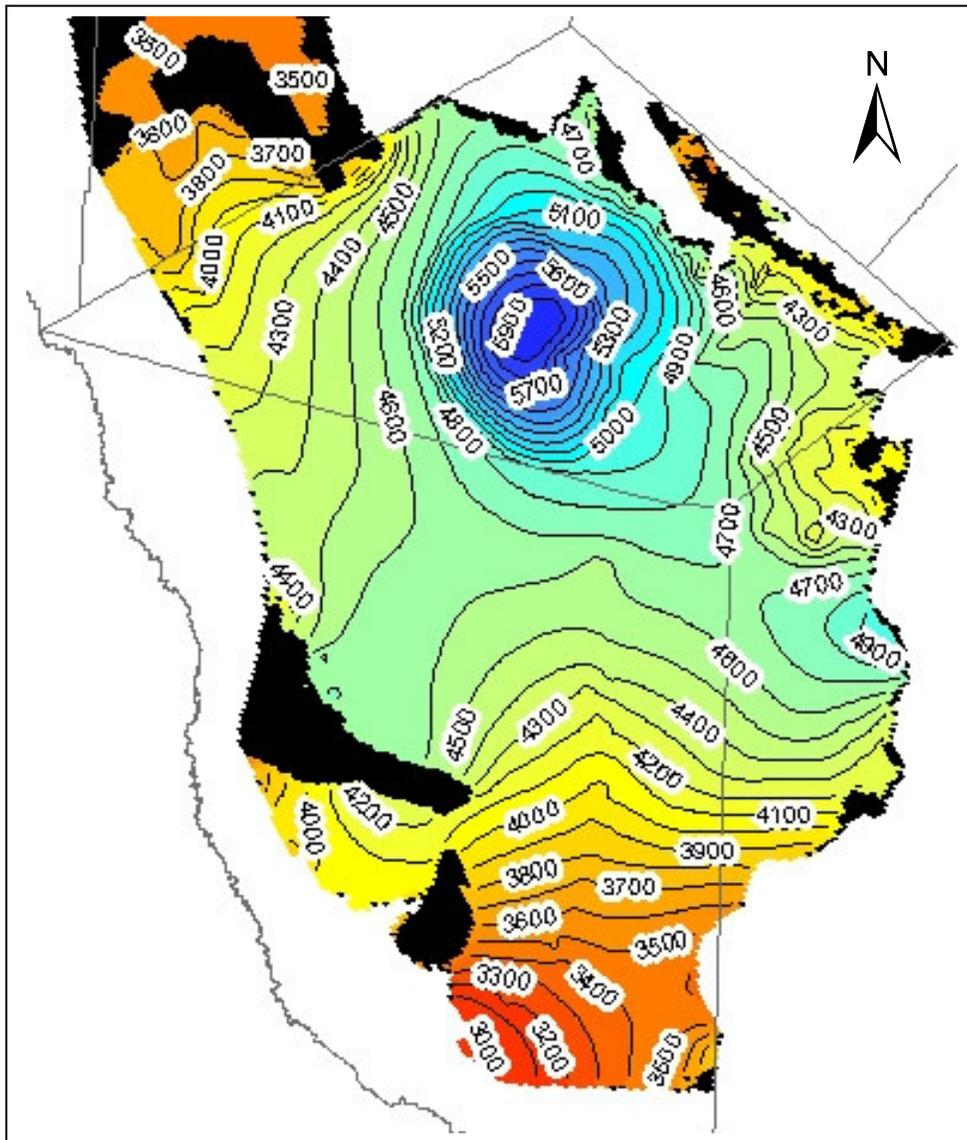
Figure 10. Water levels in the Igneous aquifer after 50 years of pumping using the 2000 estimated pumpage with average recharge. Contour interval is 100 feet. Dry model cells in the model run are shown in black.
