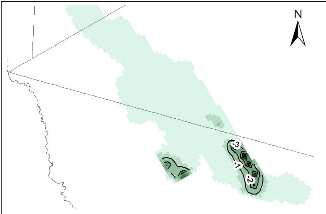
Figure 7. Difference in drawdowns in the Salt Basin aquifer after 50 years of pumpage when using average compared to drought-of-record recharge. The difference is minimal in most of the study area. The only locations with significant differences are at discrete points where alluvial fan/streambed recharge is added to the Salt Basin aquifer. Contour interval is 1 foot.
