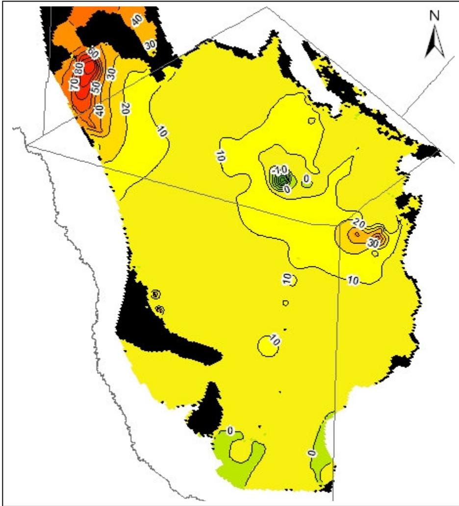
Figure 12. Drawdowns in the Igneous aquifer after 50 years of pumping using the 2000 estimated pumpage with drought-of-record recharge. Contour interval is 10 feet. Areas in green are showing recovery (and therefore have negative drawdowns); areas in yellow and orange are showing drawdown. Dry model cells in the model run are shown in black.
