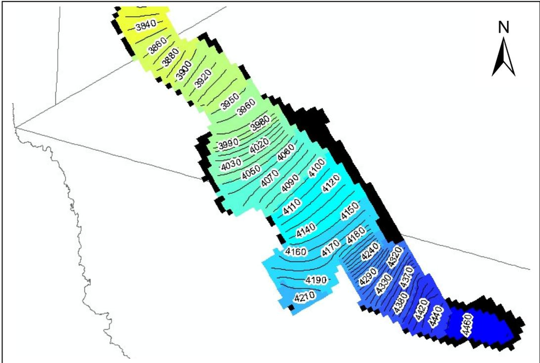
Figure 4. Initial water levels in the Salt Basin aquifer in the year 2000. Contour interval is 10 feet. Black areas are where the GAM showed the aquifer is dry.
