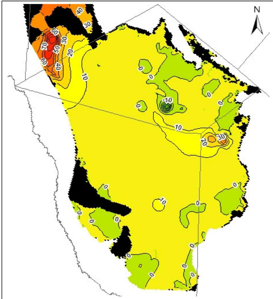
Figure 11. Drawdowns in the Igneous aquifer after 50 years of pumping using the 2000 estimated pumpage with average recharge. Contour interval is 10 feet. Areas in green are showing recovery (and therefore have negative drawdowns); areas in yellow and orange are showing drawdown. Dry model cells in the model run are shown in black.
