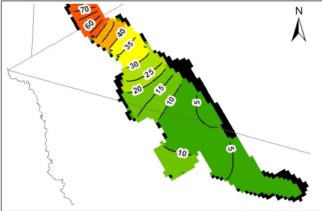
Figure 6. Drawdowns in the Salt Basin aquifer after 50 years of pumping using the year 2000 estimated pumpage with average recharge. Contour interval is 5 feet. Dry model cells in the model run are shown in black.
