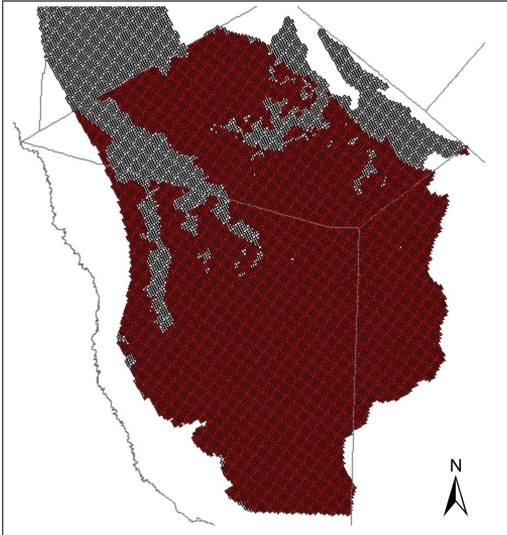
Figure 8. Extent of the Igneous aquifer in the GAM. Model cells in red are active cells that contain pumpage in 2000. Model cells in white are active cells without pumpage. The scale of this figure makes it difficult to see individual model cells.
